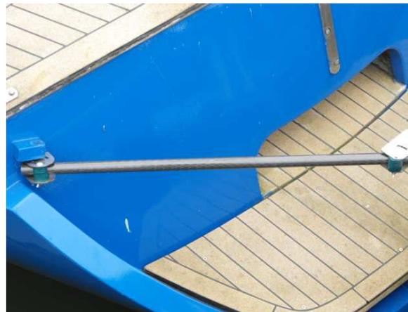
087.11 Add the boat clamps to both of the the ends of the tube using tube clamp halves, m6x50 mm mushroom head square neck bolts and m6 wing nuts.
