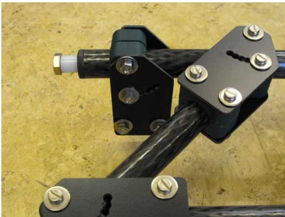
087.22 Connect the second set of stepped hinges to the 550 mm rear tube where there is room:
