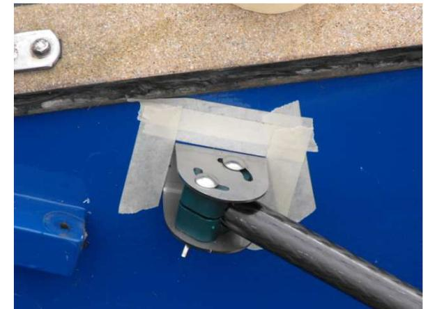
087.12 Rotate the combined boat clamps so the point where it meets the transom is flush.
