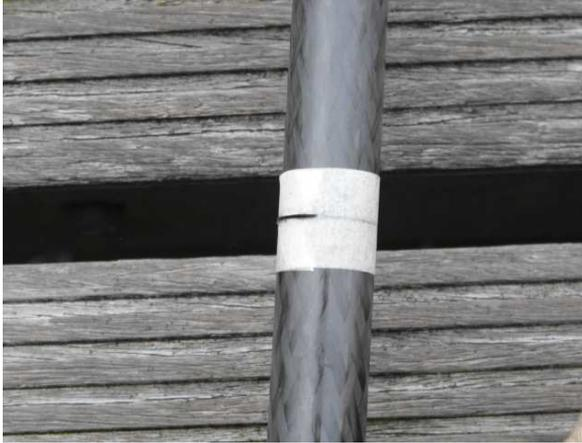
087.25 ...Mark the length the mounting tube needs to be and cut to this length as described earlier in this manual
