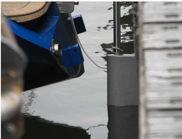
087.10 Check that the pendulum rudder is far enough behind the transom to move freely from side to side. ALSO CHECK if it does not touch any part of the boat BELOW THE WATER LINE!
