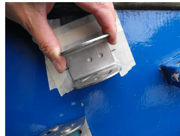
087.15 Slide the system away from the position and hold an unused boat clamp in the vacated spot....
