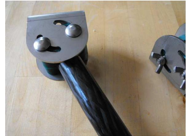
087.21 add the remaining 2 mounting tubes to the assembled boat clamps
