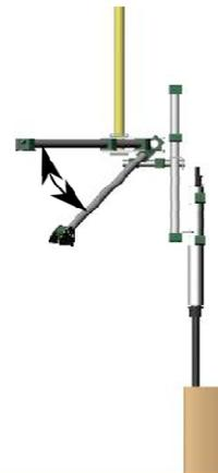
087.23 ...The aim is to get the bottom mounting tubes at a 30-90 degree angle with the horizontal.
