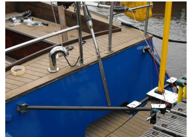
087.18 Connect the boat clamps to the transom with bolts and nuts (not included)
