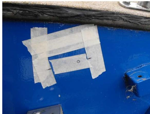
087.17 Also do this on the other side, then drill the holes in the marked position
