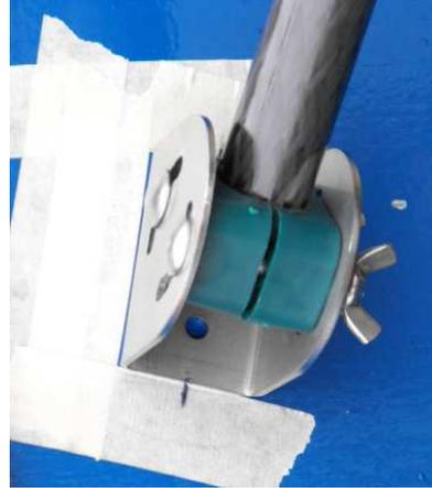
087.26 connect the tube to the stepped hinge clamp and move the face of the boat clamp so it is flush with the transom.
