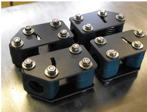
087.4 Assemble 4 sets of stepped hinges, 2 left, 2 right, using tube clamp halves, m6x50 mm screws, m6x18 mm washers (on both sides of the stepped hinges) and m6 nuts.
