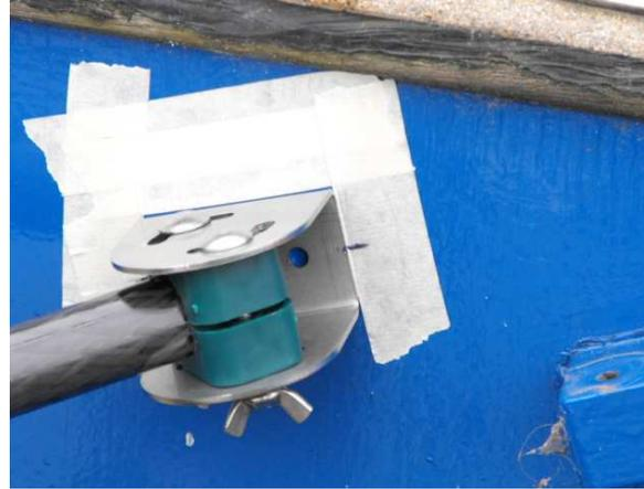
087.14 Mark the 2 small notches on each boat clamp
